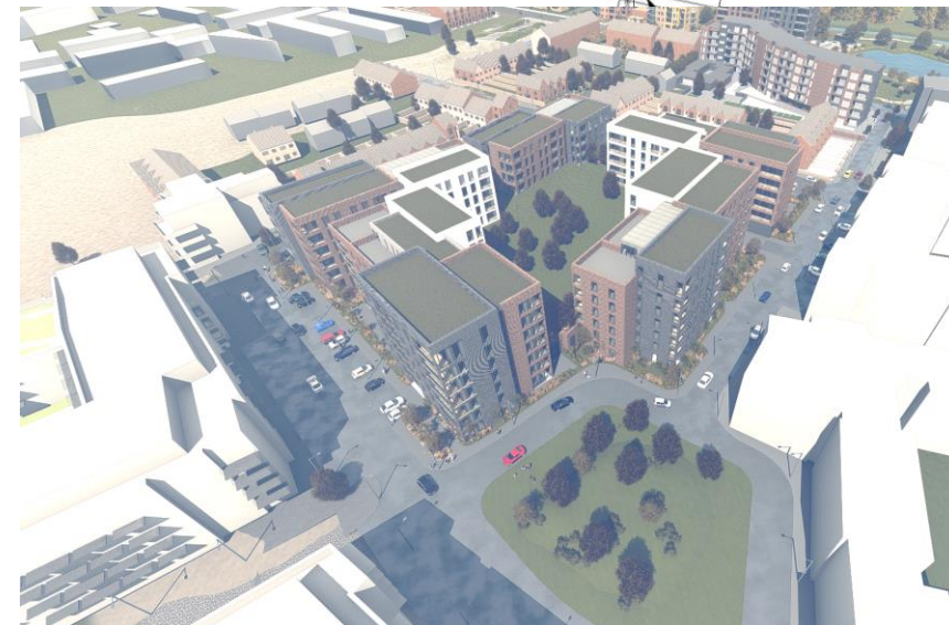
Stage 03 Proposal 5 Separate blocks – 66% Dual Aspect 5 Cores – 50 Apartments per floor (10 per Core)
