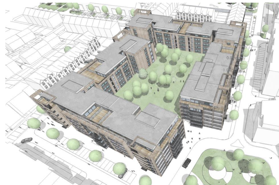
Stage 01 Proposal 2 Large L shapes blocks – 35% Dual Aspect 8 Cores – 56 approx Apartments per floor (7 per Core)
